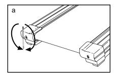
b. If the walking belt slips when walked on, first remove the key and UNPLUG THE POWER CORD. Using the allen wrench, turn both rear roller bolts clockwise 1/4 of a turn. When the walking belt is correctly tightened, you should be able to lift each side of the walking belt 3 to 4 inches off the walking platform. Be careful to keep the walking belt centered. Plug in the power cord, insert the key, and walk on the tread-
